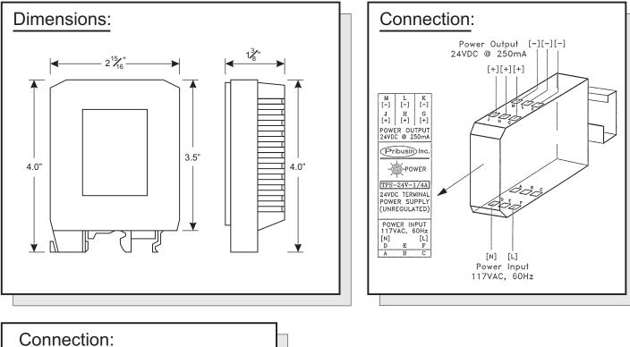
Connection: Field Connections G,H,J [N]-D -[+] [N] [+] POWER POWER POWER POWER OUTPUT INPUT OUTPUT 117VAC, INPUT 24VDC. @ 250mA 60Hz [-] [L] [L] -F K,L,M - [ -- ] TPS-24V-1/4A 24VDC POWER SUPPLY
